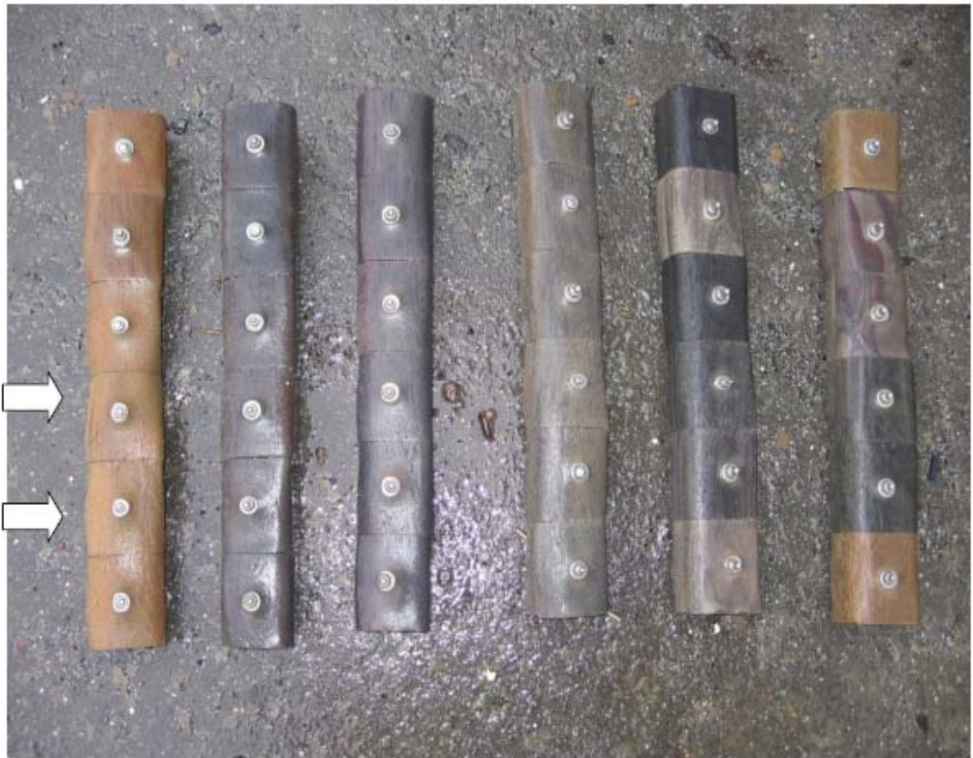
Photograph 14 Blocks at the end of 80,000 revolutions. Arrows show the rounded arrises as a result of wear.
